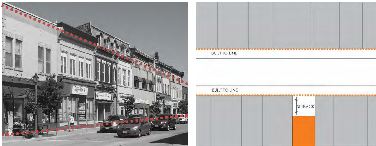
Plate 1: Maintain the setback of properties along the streetscape façade that forms a consistent and unified heritage fabric along the street wall, as noted in the top left illustration. Deep setbacks from the street wall should be avoided, as noted in the top right illustration. If a setback exists, consider adapting this for a new infill project or an urban park.
