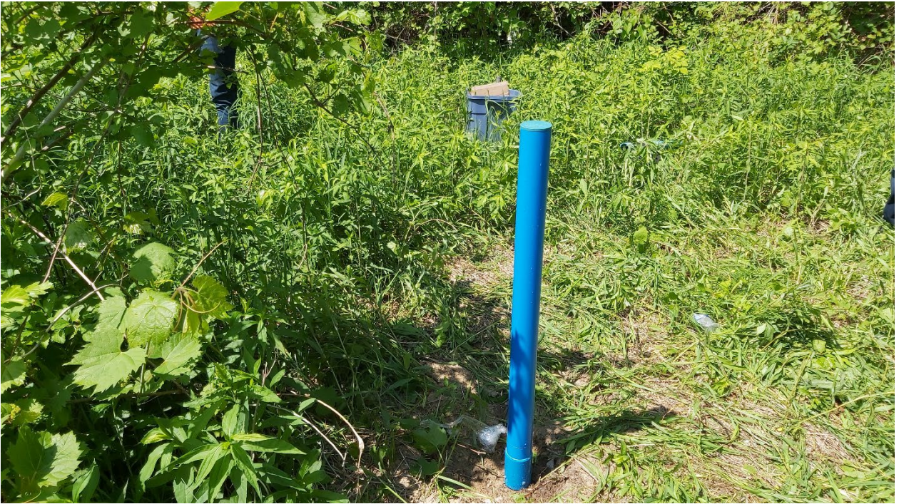
Photo 25 – Slope Inclinometer SI-01, after completion of repair, looking west (May 31, 2022).
