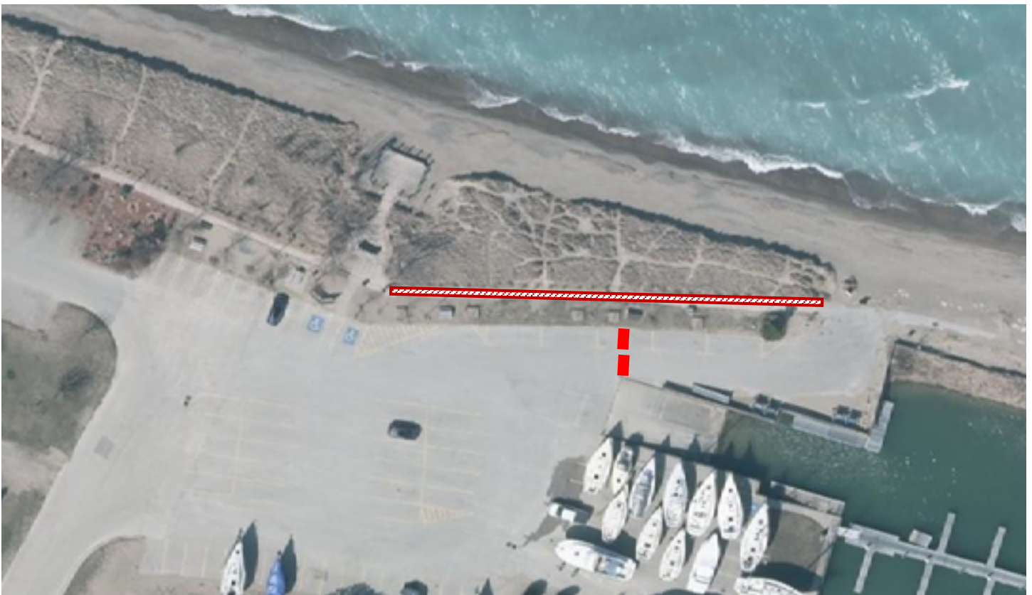
Bollard location to limit vehicles from parking in emergency parking allocation.
