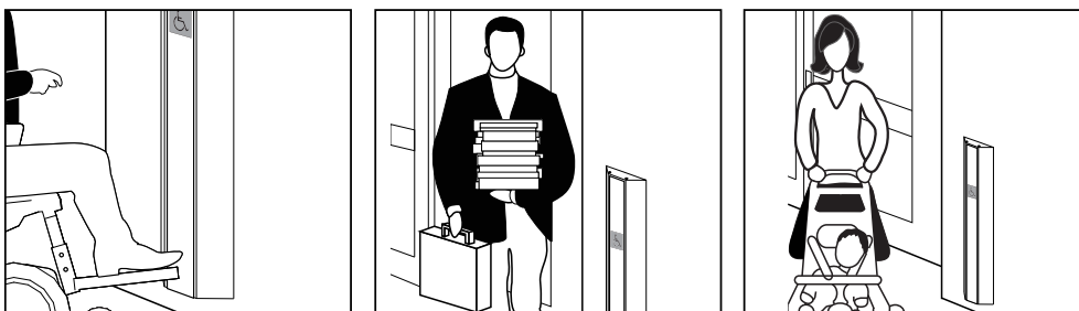
Figure 40: Example of Control for Power Door Operator Promoting Universal Use
