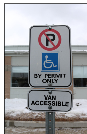
Example of Type A “VAN ACCESSIBLE” vertical signage, City of London.
