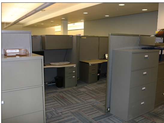
City of London Office: Example of required clear entry width into accessible workstation (e.g., with flexible / adaptable systems furniture).
